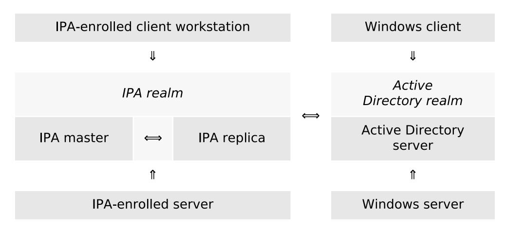
The arrows show the direction of the enrollment / trust and authentication operations. Communication can place from any client to any server.
